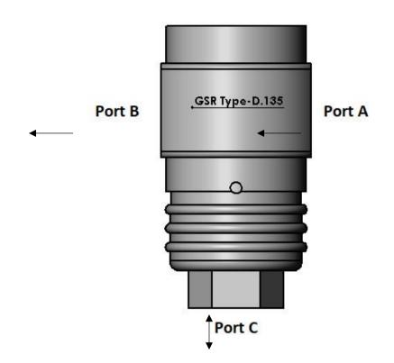
The internal mechanism (Spool arrangement et al) of the GSR Valve regulates the flow and pressure at Port **B & C** in accordance with the Load Pressure at **Port C**. This internal assembly ensures that the **Ports B** is always approx. **100kPa** above the Slurry Pump's discharge pressure.
