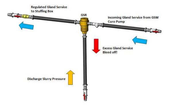
The GSR Valve consists of both; a self-regulating flow control device and a self-regulating pressure control device. The GSR Valve has three ports for flow entry and discharge:
